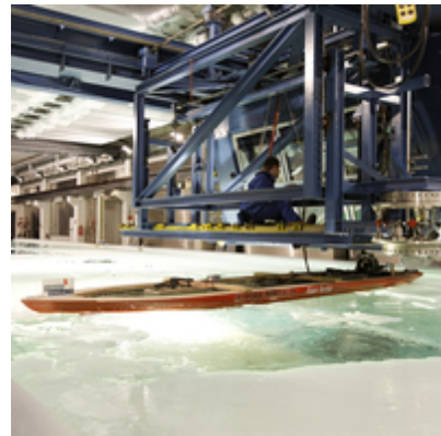
Ice model tests by Aker Arctic Technology in Helsinki, Finland Photo: AWI/Jan Meier, Bremen
