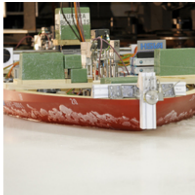
Ice model tests by Hamburgische Schiffbau-Versuchsanstalt (HSVA) in Hamburg, Germany Photo: AWI/Jan Meier, Bremen
